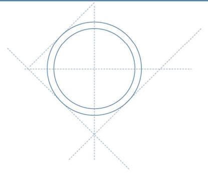
The bevelled side of the orifice plate is the downstream side.
